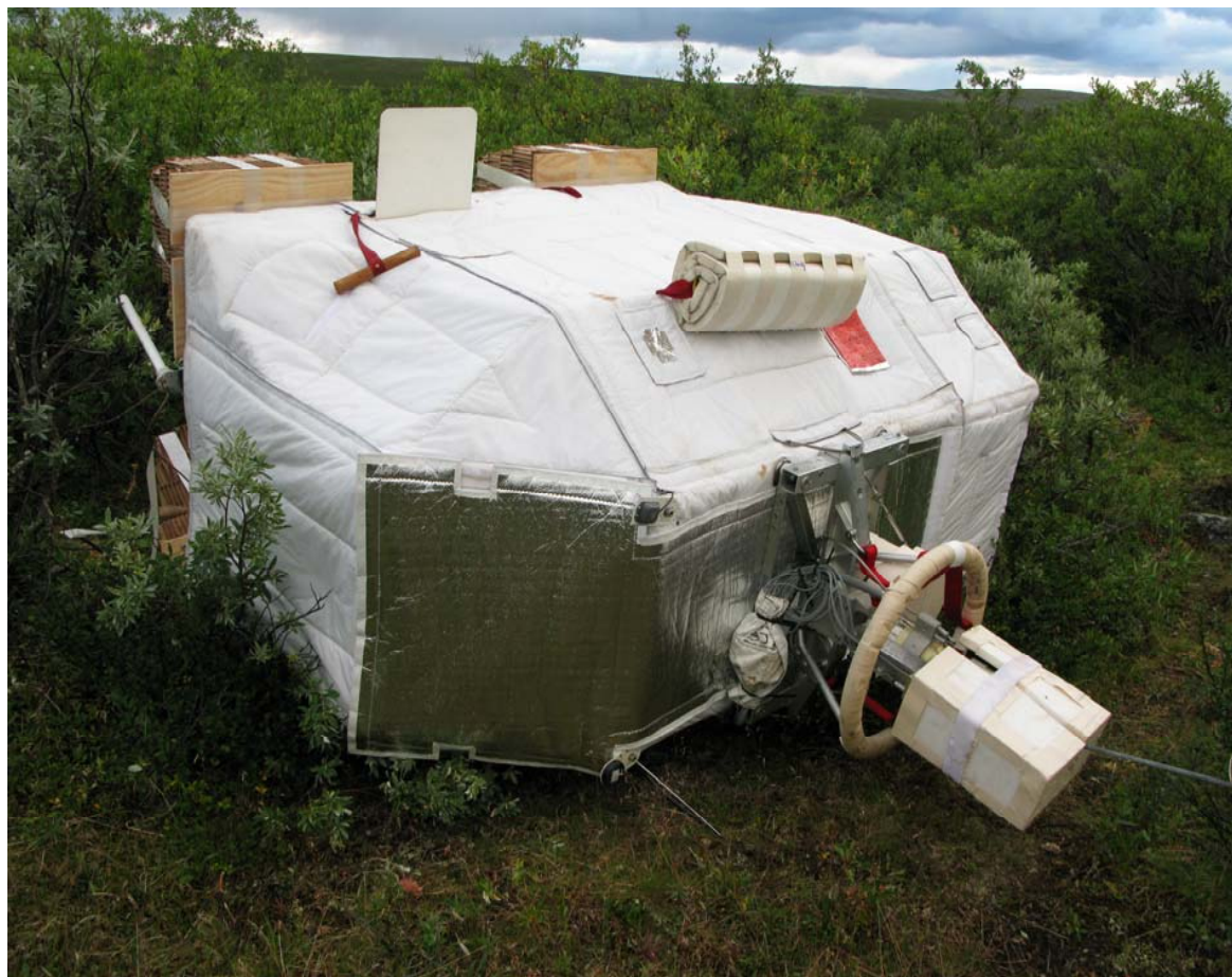
SWIR-balloon payload on the recovery site. The azimuth control system of the gondola (pivot) is clearly seen on the top of the gondola (lying on its side in this case)
